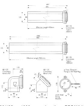
80/125 1000mm PPS/White length Galvanised Concentric Flue **PPS/White** 80/125 500mm length Galvanised Concentric Flue 80/125 PPS/White Galvanised 90 degree elbow 80/125 PPS/White Galvanised 45 degree elbow 125mm Wall Fixing Clamp
