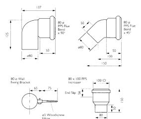
80mm 1000mm PPS flue pipe 80mm PPS 45 degree PPS Elbow 80mm PPS 45 degree connector 80mm Wall Fixing Clamp 80mm – 100mm increaser
